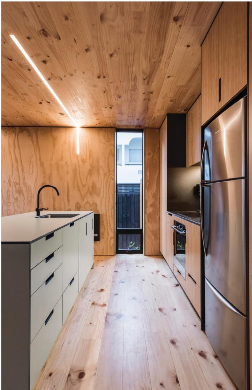
Compact laminate has been used for the custom designed kitchen island and vanities. This material offers a very durable finish and is impregnated with silver to maintain a hygienic surface. The solid block of colour offers a counterpoint to the heavy use of timber. The black exposed edges to the laminate mimic the black negative details to the wall linings.
